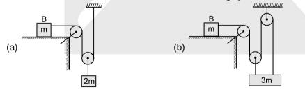
**E-7.** Find out the mass of block B to keep the system at rest :  $(g = 10 \text{ m/s}^2)$
