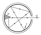
It consists of an enclosure with a small opening which is painted black from inside. The opening acts as a perfect black body. Any radiation that falls on the opening goes inside and has very little chance of escaping the enclosure before getting absorbed through multiple reflections. The cone opposite to the opening ensures that no radiation is reflected back directly.
