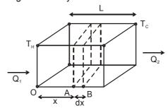
Consider a slab of face area A, Lateral thickness L, whose faces have temperatures  $T_H$  and  $T_C$  ( $T_H > T_C$ ). Now consider two cross sections in the slab at positions A and B separated by a lateral distance of dx. Let temperature of face A be T and that of face B be T +  $\Delta T$ . Then experiments show that Q, the amount of heat crossing the area A of the slab at position x in time t is given by
