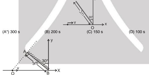
In the figure shown the line 'OA' is normal to the mirror passing through the end point A. By ray diagram it can be shown that when the insect is to the left of 'O' all its reflected rays will be towards right of 'O' so it cannot see its image because rays are not reaching it. when the insect is to the right of 'O' its reflected rays will be on both sides of the insect that means the insect will be in the field of view of its image. So it can see its image.
