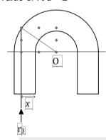
Let the intensity of beam be  $I_0$ . Flux entering through glass slab will be  $dI_0$ . Assume that any light ray up to distance x from the edge BC undergoes at least one total internal reflection. Then the flux going through at least one total internal reflection will be  $(d-x)II_0$ . Also
