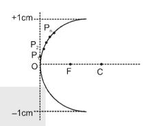
36. A symmetrical converging convex lens of focal length 10 cm & diverging concave symmetrical lens of focal length –20 cm are cut from the middle and perpendicularly and symmetrically to their principal axis. The parts thus obtained are arranged as shown in the figure. Find the focal length (in cm) of this arrangement
