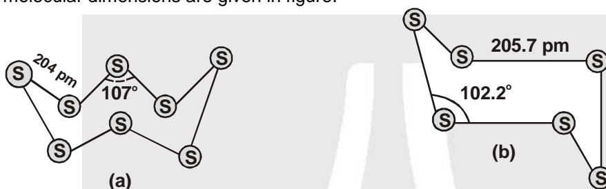
Fig. : The structures of (a) S_8 ring in rhombic sulphur and (b) S_6 form
