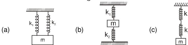
**Ans.** (a)  $2\pi\sqrt{\frac{m}{k_1+k_2}}$ ,  $k_{eq.} = k_1 + k_2$ ; (b)  $2\pi\sqrt{\frac{m}{k_1+k_2}}$ ,  $k_{eq.} = k_1 + k_2$ ; (c)  $2\pi\sqrt{\frac{m(k_1+k_2)}{k_1k_2}}$ ,  $k_{eq.} = \frac{k_1k_2}{k_1+k_2}$
