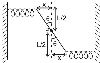
$$\text{Torque about P} = (kx) \frac{L}{2} + (kx) \frac{L}{2} = kxL \left(\theta = \frac{2x}{L}\right)$$
