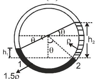
(b) When liquids are slightly disturbed by an angle  $\beta$ . Net restoring pressure  $\Delta P = 1.5 \rho g h + \rho g h$  This pressure will be equal at all sections of the liquid. Therefore, net restoring torque on the whole liquid.
