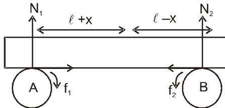
Let  $N_1, N_2$  and  $f_1, f_2$  are Normal and friction force at Point A and B
