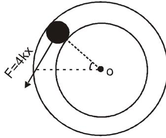
Spring in lower side is stretched by  $2x$  and on upper side compressed by  $2x$ . Therefore, each spring will exert a force  $2kx$  on each ball.
