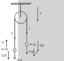
Force on  $m_1$  and  $m_2$  due to electric field =  $Q_1E$  and  $Q_2E$  downward Let acceleration of both masses is 'a' as shown in figure:
