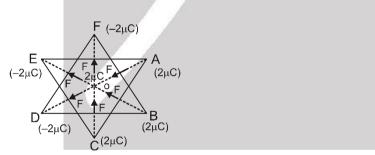
The given figure shows force diagram for charge at O due to all other charges with  $r = \frac{10}{\sqrt{3}}$  cm
