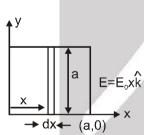
flux through differential element  $d\phi = E_0 x$  a dx.
