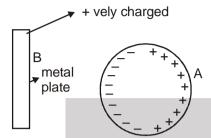
The given diagram shows induction on sphere (metallic) due to metal plate.
