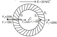
$F_1$  = Force on Q due to induced charge on  $S_1$  = 15 N,
