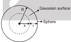
Let us construct a Gaussian surface at distance r from surface of sphere inside it (as shown dotted in figure)
