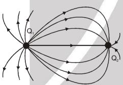
From the diagram, it can be observed that Q<sub>1</sub> is positive and Q<sub>2</sub> is negative.
