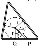
Let us consider a small length of rod at position P on one of the sides of the triangle; let it subtend an angle  $\Delta \phi$  at the incentre (see figure). Its distance from the incentre is r/cos  $\phi$ . Its small length  $\Delta x$  can be found by noting that P is a distance  $x = r \tan \phi$  along the rod from the fixed point Q and so  $\Delta x = (r \Delta \phi) / (\cos^2 \phi)$ . Consequently the charge it carries is
