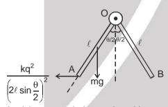
Applying torque balance about hinge point O.
