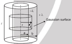
Using Gauss's law for Gaussian surface shown in figure.
