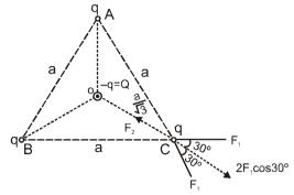
Equating the forces on charge q placed at point 'C' we see,
