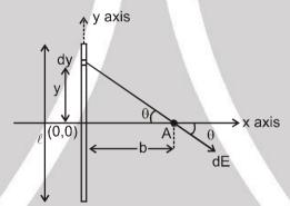
Charge on the element  $dy = \frac{q}{\ell} dy$
