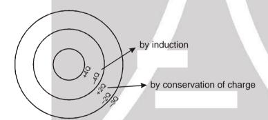
Given diagram shows the charge distribution on shells due to induction & conservation of charge.
