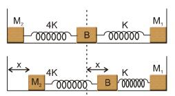
As springs and supports  $(m_1 \text{ and } m_2)$  are having negligible mass. Whenever springs pull the massless supports, springs will be in natural length. At maximum compression, velocity of B will be zero.
